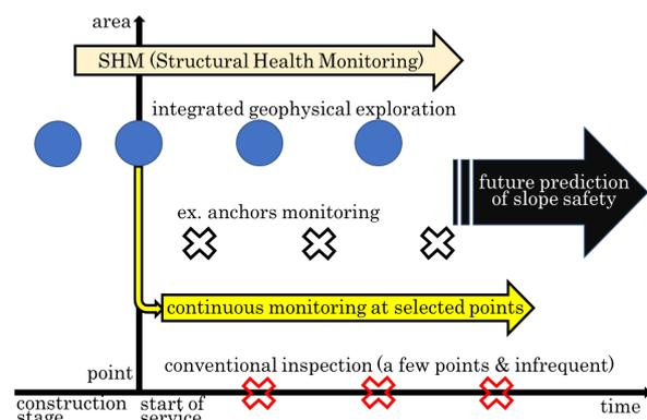
Fig. 1 SHM and development of some challenging monitoring system.
